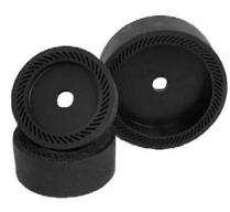
Angled expansion slots through the heavy rubber rim allow the drum to expand when rotated; thereby locking the belt in place. Belts can be quickly changed by stopping the machine, slipping of the old one and sliding on the new. In use, the resilient drum surface flexes to the gemstones contour to quickly remove grinding flats. The convex shaped drum provides the cutting action necessary to remove scratches. Sold without belt.
