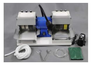
This Cabbing Grinder Machine made by our company, with 5/8" shafts and ball bearing. With 1" alloy aluminum shaft sleeve suit for 1\_" hole wheel and expandable drums, 7pcs Aluminums Spacers and Flanges (Suit for two type popular wheel) and locknut It also has a 1/4 HP Thermal protected ball bearing motor, the Hood process by Alloy aluminum and powder coating, The Cover has two U-Slot for easy remove, We also supply a adjustable drip water
