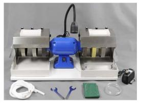
This Cabbing Grinder Machine with 1"stainless steel shafts and ball bearings,7pcs Aluminums Spacers and Flanges and locknut It also has a 3/4HP Thermal protected ball bearing motor, the Hood process by 304 stainless steel. We also can supply a adjustable drip water system with 8 shut off valves for each wheel. The shaft is tapped for a 1/4-20 spin-on polish head at right ends and tapped for a 1/2" Aluminum lap or Diamond
