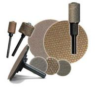
Flexible Diamond bands and discs are made from a two-ply polyester backing film evenly coated with diamond filled nickel plated dots. These flexible diamond bands have been designed and developed for light grinding, shaping and polishing applications with contours and hard to reach areas on hard materials, such as granite, marble, natural stone, engineered stone, glass, ceramics and hard metals. Use wet or dry. Use to grind, sand and smooth on these materials: glass, stone, wood,
