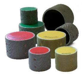
M14 fitting, flexible diamond vanity drums with central water feed for wet grinding and polishing internal cutouts in glass. The diamond vanity drums are color coded M60 green, M120 black, M200 red and M400 yellow for easy grade identification.
